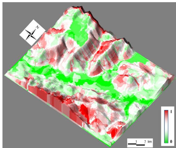
**Fig. 11.** Aggregated landslide susceptibility map (perspective view) using the Arithmetic Mean method for the Kaixian study area. Color: 0 – not susceptible at all to landslide occurrence. 1 – extremely susceptible to landslide occurrence.
