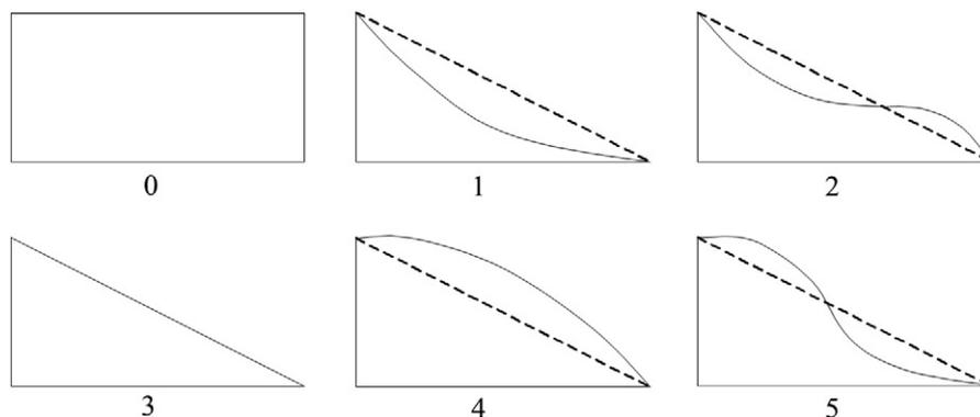
**Fig. 10.** Classification of slope shapes in the study area. 0: Flat area. 1: Concave hillslope. 2: Upper concave, lower convex hillslope. 3: Straight hillslope. 4: Convex hillslope. 5: Upper convex, lower concave hillslope.
