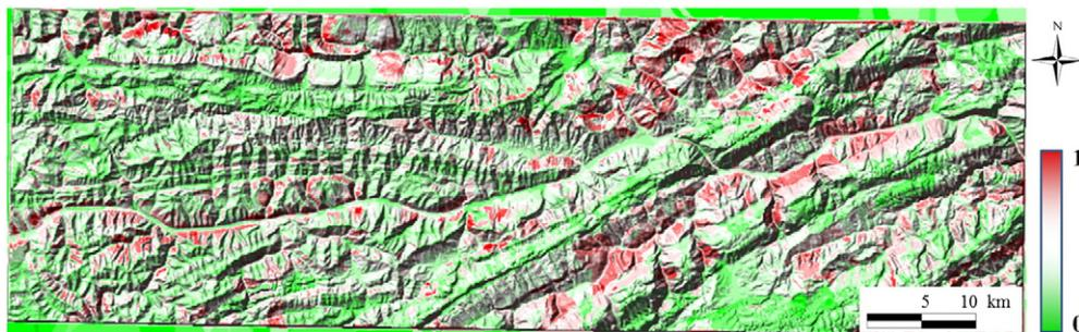
**Fig. 13.** Aggregated landslide susceptibility map using the Arithmetic Mean method for the Three Gorges study area.
