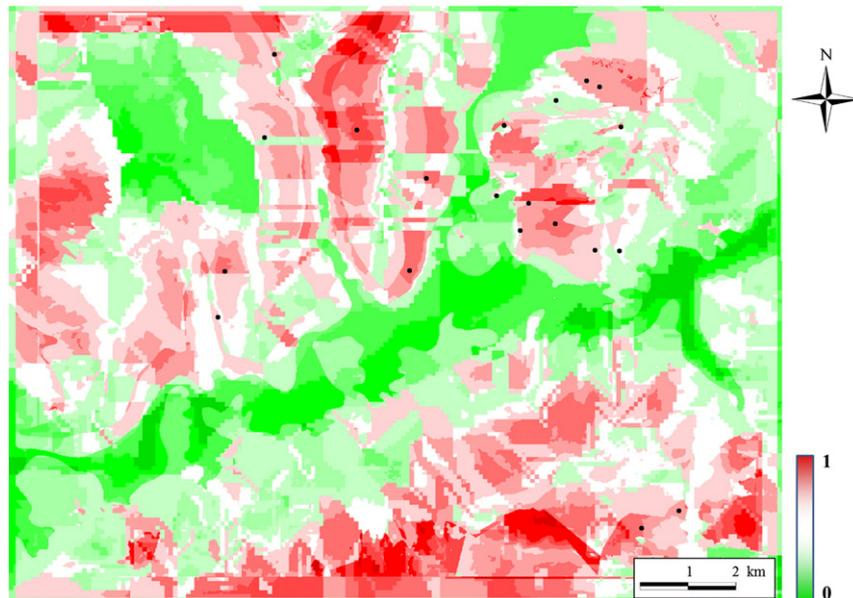
**Fig. 12.** Aggregated landslide susceptibility map with landslide points for the Kaixian study area. Black dots represent the locations of observed landslides.
