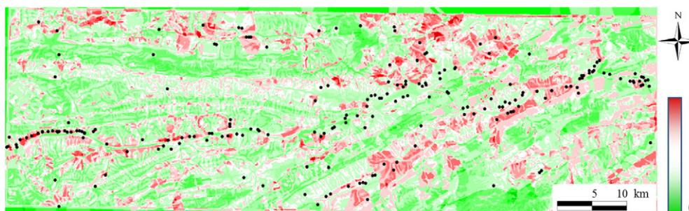
Fig. 14. Aggregated detailed landslide susceptibility map with landslide points for the Three Gorges study area. Black dots represent the locations of observed landslides.
