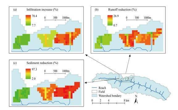
Fig. 4 Distribution of infiltration increase, runoff reduction and sediment reduction after BMPs implemented.
