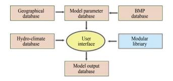
Fig. 2 Structure of the modeling system (SEIM).
